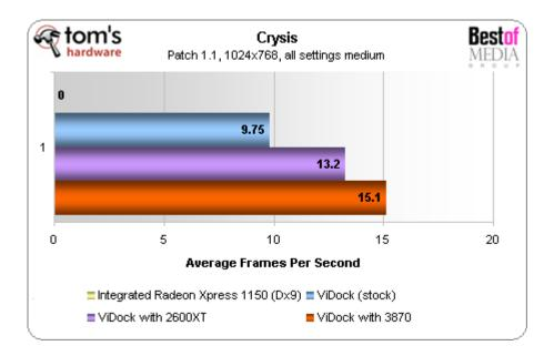
At the shader intensive medium settings, the 3870 takes its rightful place at the head of the pack. But it's important to note that the 3870 can't even muster enough power to play Crysis at medium settings at 1024x768, again because of the ExpressCard bus's relatively low bandwidth.
