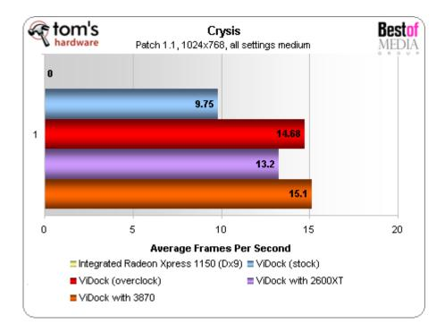
At the shader-intensive medium settings, we see the 3870 has retaken the lead, but it is very closely followed by the overclocked 2600 PRO, which continues to outperform the 2600 XT!
