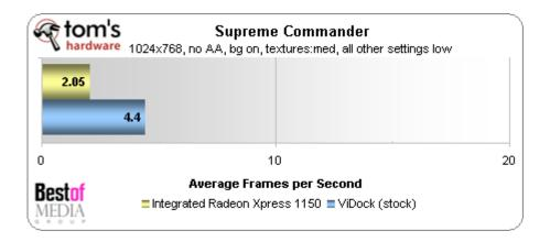
Ouch! While the ViDock managed to double the frame rate of the integrated graphics, it's somewhat of a pyrrhic victory: 4.4 frames per second is far from playable. While Supreme Commander is a CPU-dependent game, it should have been able to muster better frame rates than this with a dual-core Athlon, so we can't give the ViDock a lot of credit here.œ
