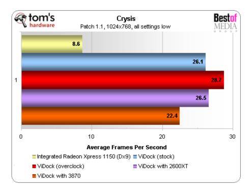
The results are puzzling to say the least: the overclocked 2600 PRO managed to best both the 2600 XT and the 3870. While the 3870 was clearly somehow stunted in this benchmark, what doesn't make sense at all is how the 750 MHz core / 550 MHz memory on the overclocked 2600 PRO beat out the 800 MHz core / 700 MHz memory on the stock 2600 XT. The chipset on the two cards should be identical.
