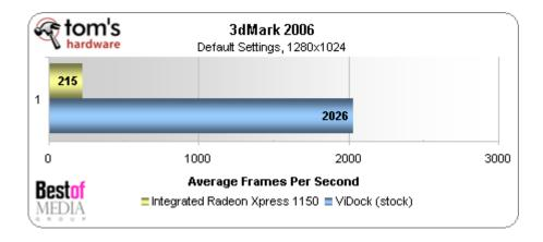
We'll start with the synthetic gaming test 3dMark 2006, where we immediately see a dramatic improvement in performance: the ViDock provides a tenfold increase in <u>3D gaming</u> speed according to this benchmark! At this stage, it doesn't look like the limitation of bandwidth from the ExpressCard bus is going to slow the ViDock down much. But 3dMark can be deceiving, so let's have a look at an actual game title, such as Prey.
