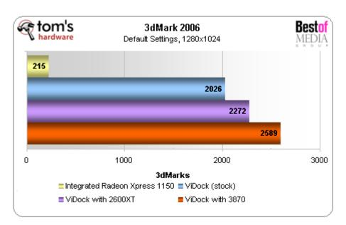
3dMark shows us the ExpressCard bandwidth bottleneck as clear as day. The Radeon 3870 should be getting scores many times that of the 2600 PRO in the stock ViDock, but instead we saw only a subtle increase in performance. The 2600 PRO is looking like a good match for the slow ExpressCard bus.
