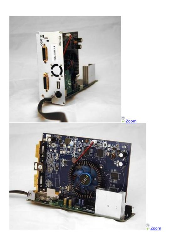
At its heart, the ViDock is an ExpressCard-to-PCIe adapter, as we can see when the card is removed.
