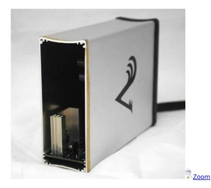
With the covers off, the main circuit board and <u>graphics card</u> slid out easily, showing us the man behind the curtain: the Radeon 2600 PRO 512MB, in this case, an HIS branded card.
