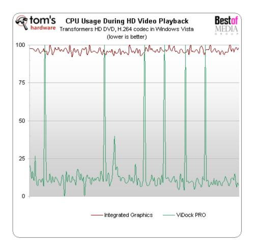
When it comes to HD <u>video playback</u> at the 1920x1080 resolution, the ViDock Pro is absolutely invaluable. Since the integrated Radeon Xpress 1150 has no HD acceleration, CPU utilization stayed close to 100%, yet <u>playback</u> still stuttered and was unwatchable! Contrast this with the ViDock, which allowed for HD acceleration on the GPU, removing the lion's share of the <u>decoding</u> and lowering CPU utilization to about 10%. More importantly, <u>playback</u> was as smooth as butter.
