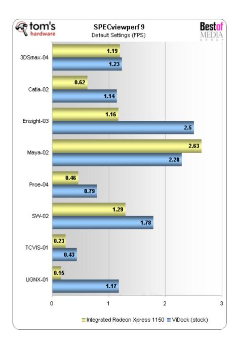
Specviewperf is a mixed bag, with the ViDock showing some impressive gains over the integrated chipset, on average, but a couple of rogue benchmarks are showing parity with the integrated chipset. It's quite possible that these particular benchmarks are favoring the integrated graphics' communication speed with the system over the ViDock's ExpressCard interface.
